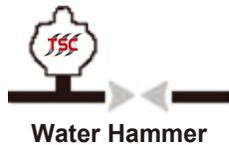
Surges in flowing systems, caused by the sudden closure of valves, pump shut-downs or start-ups, can lead to pressure build-ups that are large enough to rupture piping, piping supports and damage downstream equipment. This phenomenon, also known as water hammer, results from the sudden change of the flowing fluid's kinetic energy into pressure energy.
