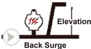
When the elevation head of a pump is high, back surges can occur from sudden pump shut-downs. Fluid then flows back and slams into the pump valve damaging it.
