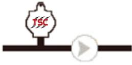
Cavitation can cause premature damage to valves, seats, plungers and other pump components. TSC Pulsation Dampeners operate as suction stabilizers, when installed on the upstream side of a pump, to help eliminate cavitation by smoothing fluid flow into the pump cylinders.
