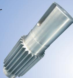
Forged **Pinion** shaft with machined gear made from high strength **ANSI 4340** steel forging for enhanced rigidity and service life.
