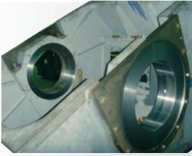
Reinforced, 36 Kip high strength, stress relieved, alloy-steel **Pump Frame** provides rigidity where its needed and longevity where its wanted. Heat treatment after fabrication removes residual stress and prevents distortion after final machining.
