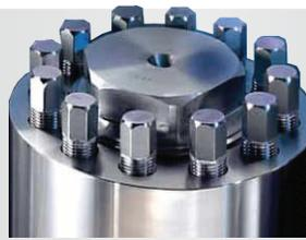
**Super Bolt & Nut** on Main Bearing cap provide significantly higher yield and tensile strength than the standard hex nut and eliminate the need for special tools not commonly available on drilling rigs.
