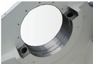
Double-reinforced, 50 Kip high strength, stress relieved, alloy-steel **Pump Frame** provides rigidity where its needed and longevity where its wanted. Heat treatment after fabrication removes residual stress and prevents distortion after final machining.
